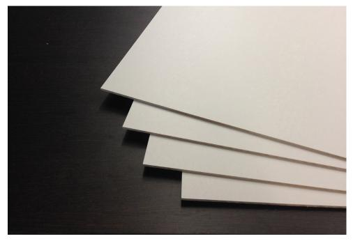
when moving them. Ensure that the sheets are positioned correctly above each other. Store in a dry interior location away from direct sunlight. Never store in an exposed or semi exposed environment.
