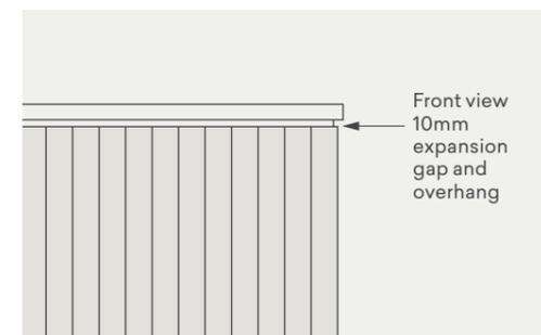
A minimum expansion gap of 10mm is required at the top and bottom edges of the Surround by Laminex panel.
