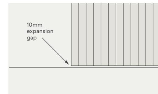
For a full run wall, ensure an allowance of 1mm expansion gap for every metre of horizontal wall covered.
