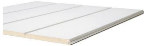
**FR\*** - Surround by Laminex is available in a MR E1 MDF Fire Resistant substrate\* with a Material Group 2 Classification. This Fire Resistant panel can be identified with the pink tongue and grey core substrate.
