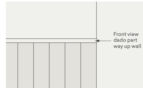
When using two different profiles side by side, apply a dado rail along the interface join between the profiles.
