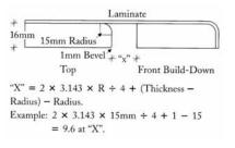
Then allow 0.5 to 1 mm for additional clearance which would give a suggested dimension at "X" of 10.5 mm.
