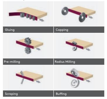
To achieve a high-quality and durable edgetape application several important processing parameters have to be considered which depend on the components used (edgetape, glue and boards), the edgebander and the ambient temperature. In order to identify the ideal conditions it is recommended that trials are carried out and that the reference values specified by the relevant manufacturer are observed.
